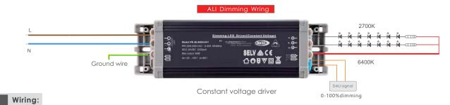
The input terminal: more than 1 m2 copper core wire.
